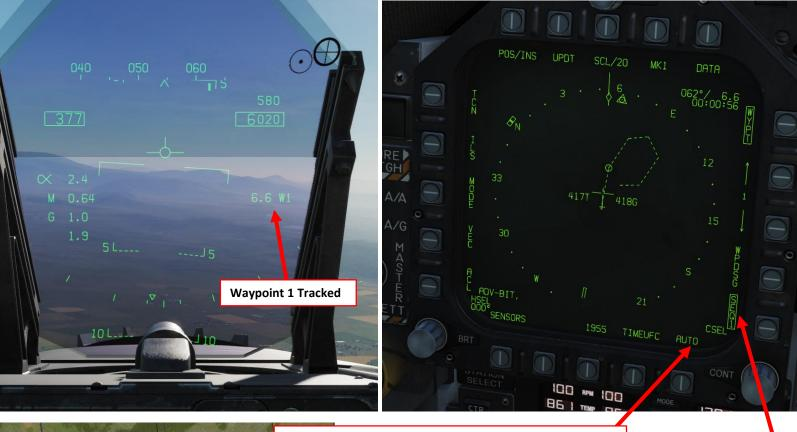
AUTO: automatic sequence steering to the next waypoint is enabled. WYPT must be selected as the navigation method
