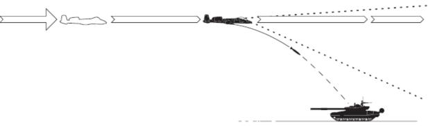
**CCRP: Continuously Computed Release Point**
