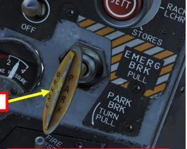
Parking Brake Engaged (Out/Pulled)
