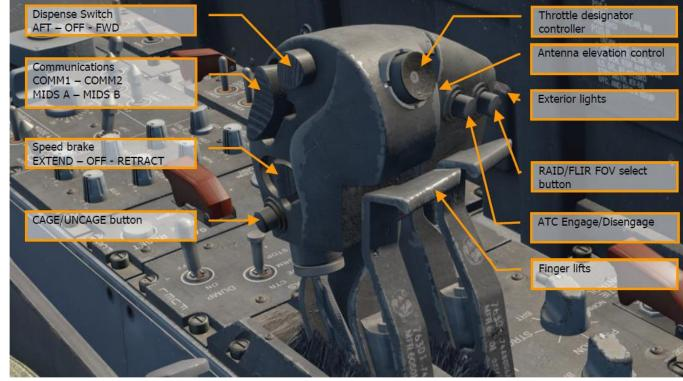
Finger lifts act as a stopper that prevents throttles from accidentally going from IDLE to OFF once engines are started. In order to shut down an engine, finger lifts are raised by pressing "0" for right throttle and "9" for left throttle.
