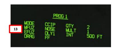
**Quantity (QTY).** Number of bombs to release, ranging from 1 to 30. When more than one bomb is selected, you must hold the Weapon Release Button down until all bombs in the salvo are released.
