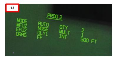
**Quantity (QTY).** Number of bombs to release, ranging from 1 to 30. When more than one bomb is selected, you must hold the Weapon Release Button down until all bombs in the salvo are released.
