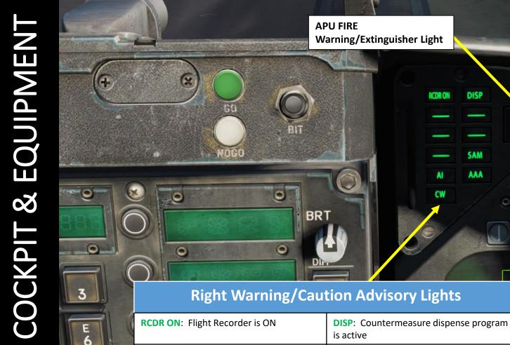
AI: Airborne Intercept (AI) Radar locked to
