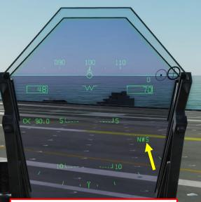
Nosewheel Steering LOW GAIN Mode (NWS)
