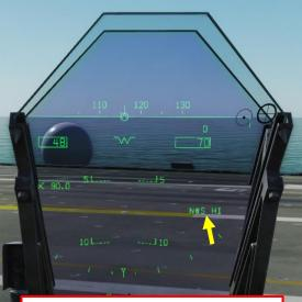
Nosewheel Steering HIGH GAIN Mode (NWS HI) NW5 (LOW GAIN): +/-16deg NWS HI (HIGH GAIN): +/-75de
